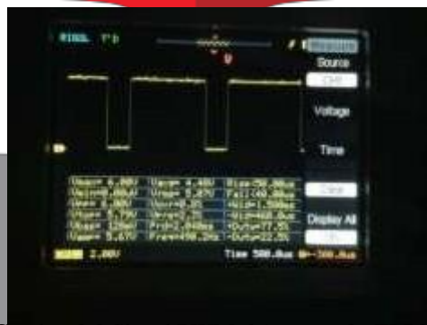
Gambar 3.3 Sinyal PWM driver mosfet TLP250
