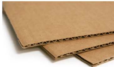
Figure.7 Corrugated board made of FBB Source: Paperboard Guide, Stora Enso Renewable Packaging
