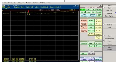
Gambar 4.3 Hasil pengukuran insertion loss 1
