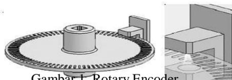
Gambar 1. Rotary Encoder
