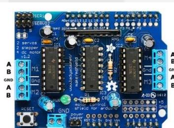
**Gambar 2.3** Motor Driver Shield L293D
