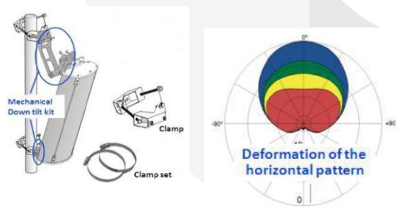
Gambar 2.2 Mechanical Tilting dan arah pancar
