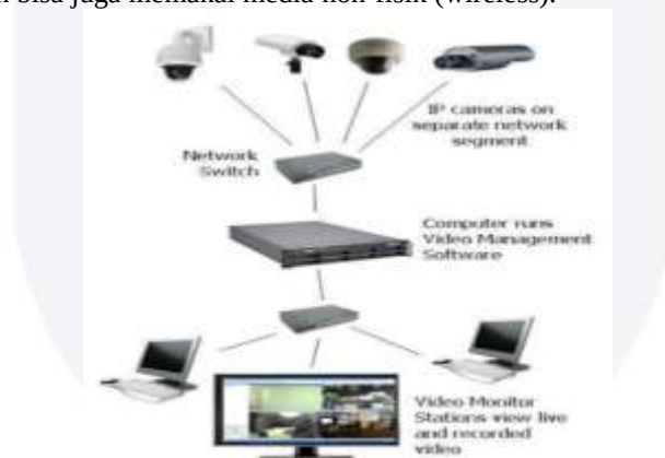
Gambar 2.2 Arsitektur IP-based Camera
