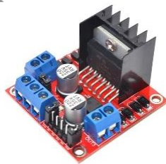
Gambar 2. Driver Motor L298N [6]
