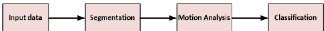
Figure 1.3: A proposed scheme of video replay attack detection on the face authentication system
