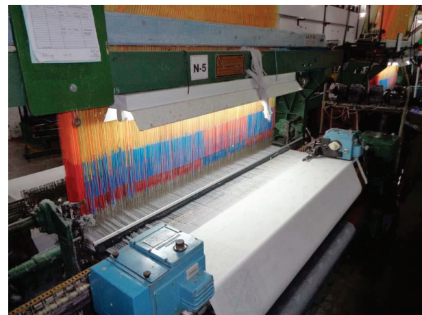
Figure 1. Jacquard Machine processing Jacquard Weaving Textile
