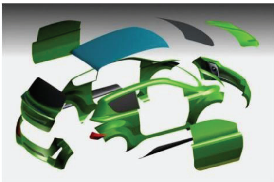
Figure15. Body exploding to exterior parts
