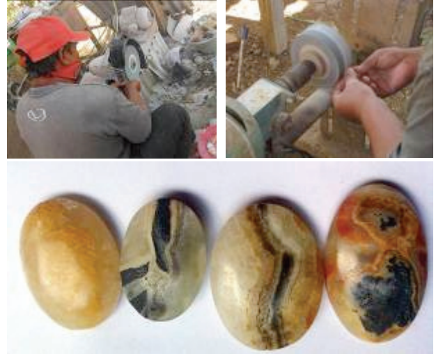
Figure 6. Experiment of cabochon cutting techniques applied to onyx. (Source: Personal document)
