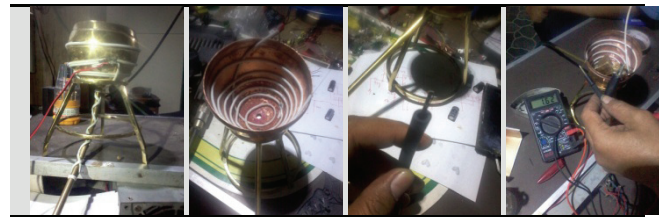
Nickelin coiling outside container Nickelin coiling at the bottom container Nickelin coiling inside cable Wax melting and current measured
