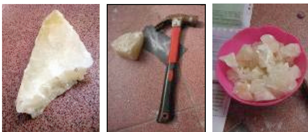
Figure 5. Experiment of rough cutting applied to onyx. (Source: personal document).
