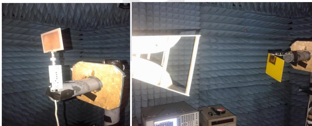
Gambar 8. Pengukuran Rectenna di ruang Anechoic Chamber
