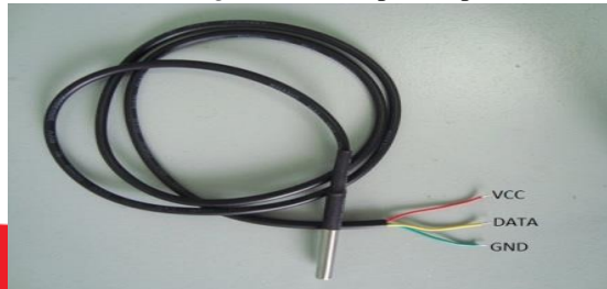
Gambar 2.2 Sensor Suhu ds18b20
