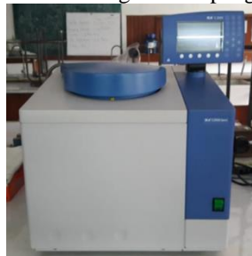
Gambar 1. Kalorimeter Bom IKA C2000 Basic .
