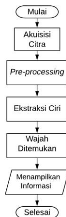
Gambar 5. Diagram Alir Perancangan Sistem Face Recognition
