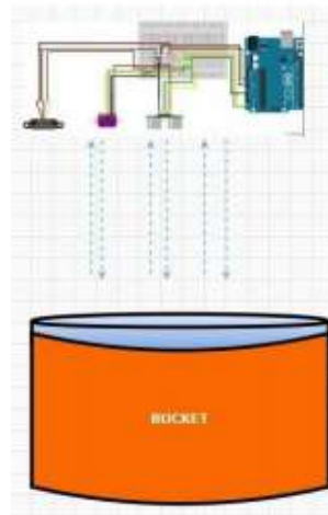
Figure 3.3 Illustration of how Arduino measurement the distance
