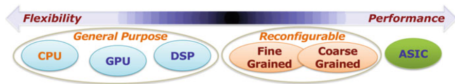
Fig. 16 Overview of the classical computing spectrum: performance versus flexibility
