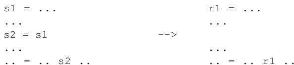
Fig. 16 Coalescing example. In the pseudocode on the left hand side, we assume that the live ranges (symbolic registers) s1 and s2 do not interfere, i.e., s2 is not accessed before the copy operation s2 = s1 and s1 not afterwards, such that the live ranges just touch each other at the copy operation. Right hand side: Coalescing s1 and s2 virtually merges both live ranges into one by forcing them to use the same physical register r1 . The copy operation is eliminated
