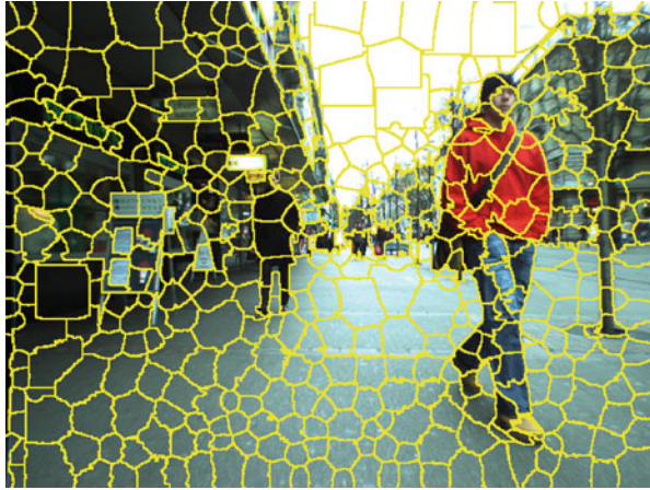
Fig. 5 Oversegmentation of the camera image, representing similar textured regions within one superpixel (orange bounds)
