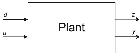
Fig. 1 A generic system to be controlled, called the plant. d is a vector of exogenous inputs; u is a vector of control inputs; y is a vector of measured outputs—available for feedback; and z is a vector of outputs that are not available for feedback
