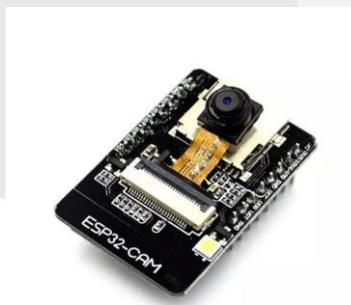
Gambar 2. 4 ESP32 CAM
