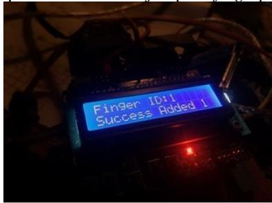
GAMBAR 4. 2 Enroll Fingerprint LCD
