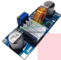
GAMBAR III. 2 Modul *Buck Converter Step Down*
