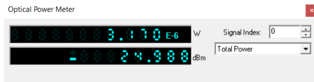
Gambar 4. 6 Hasil Power Received Terburuk Pada Link Akses Upstream
