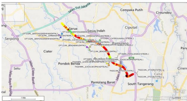
Gambar 4 Data RSRP Hasil Drive Test
