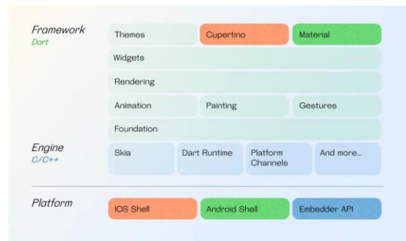
Gambar 2.3 Flutter architecture diagram[21]
