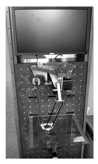
Figure 6.4 An equiplet with a delta-robot frontend
