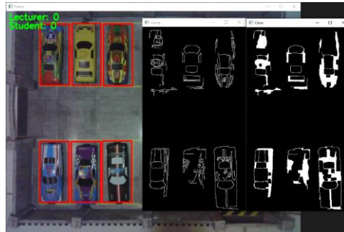
Figure 6. Canny and Closing Morphology Monitoring Results
