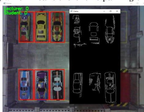
Figure 5. Canny Application Results
