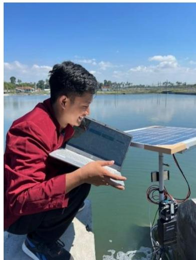
**Gambar 5. Ujicoba Alat Monitoring Tambak Udang**
