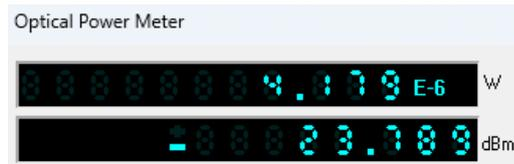
**Gambar 10** Hasil *Received Power* Terburuk Pada *Link Backhaul*
