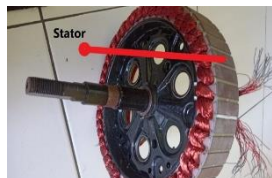
Gambar 2. 2 Desain Stator Motor Eksisting
