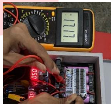
GAMBAR 13 Rangkaian Baterai 4S 2 paralel, 4 series
