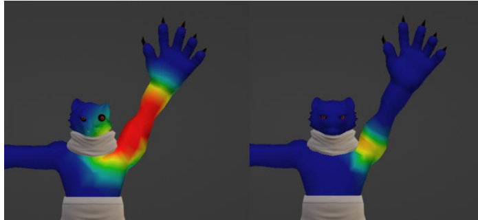
Figure 12 An example of bad skinning (left) and good skinning (right). Source: Personal Documentation (2024).
