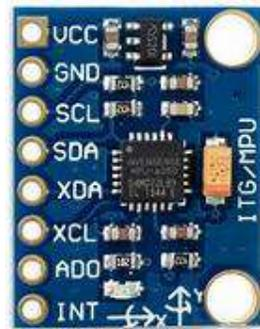
Gambar 2.2 Sensor MPU6050
