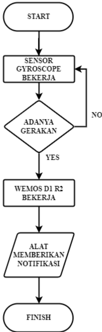
Gambar 3 4 Flowchart Sensor Gyroscope
