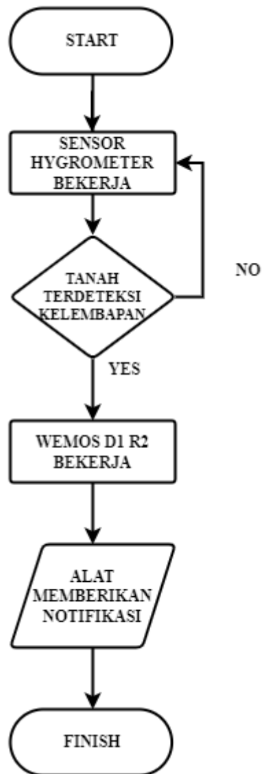
Gambar 3 5 Flowchart Sensor Hygrometer
