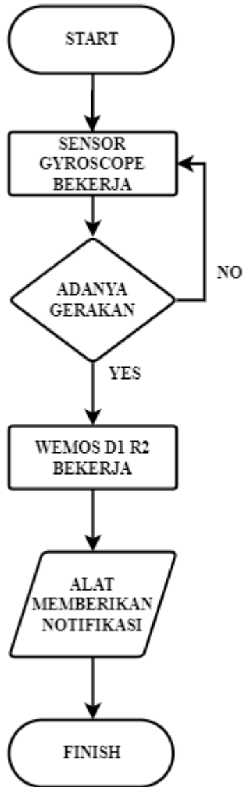
Gambar 3 4 Flowchart Sensor Gyroscope
