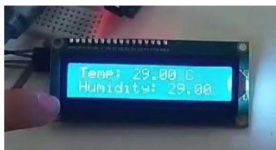
Figure 5. LCD Screen for Full System EVPLC Module Testing
