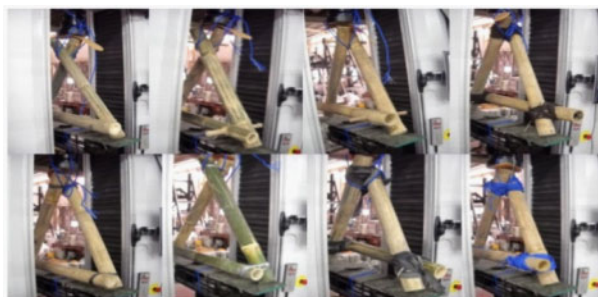
Figure 4. Manual testing images laying objects on measuring University (UTM) Eurotest type. (Source: Ahmad Nur Sheha Gunawan 2013)
