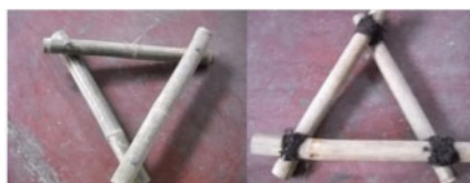
Figure 2. The test specimen to a compressive force and drag created in the form of simple construction. (Source: Ahmad Nur Sheha Gunawan, 2013)
