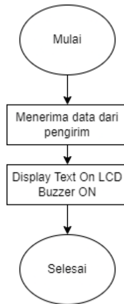
Gambar 3. 12 Flowchart Rangkain Penerima
