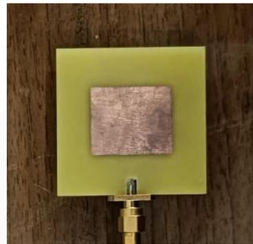
Gambar 6 (Hasil fabrikasi antenna DGS double layer)
