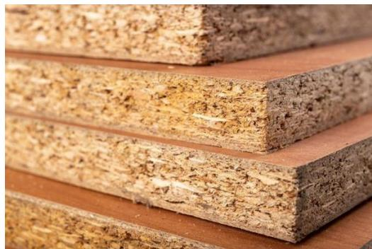
Gambar 2.10 *Particle Board*
