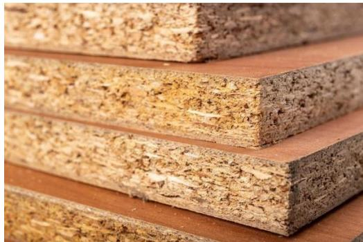
Gambar 2.10 *Particle Board*
