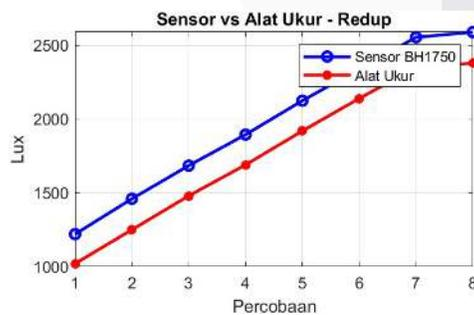
Figure 11 Grafik Sensor Vs Alat Ukur Kondisi Redup
