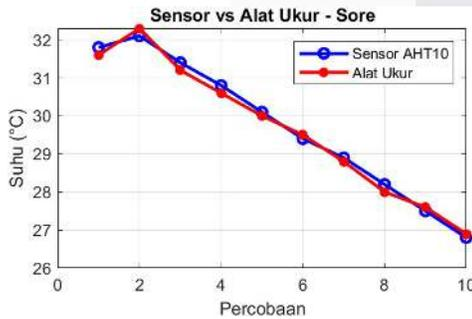
Figure 5 Grafik Sensor Vs Alat Ukur Sore
