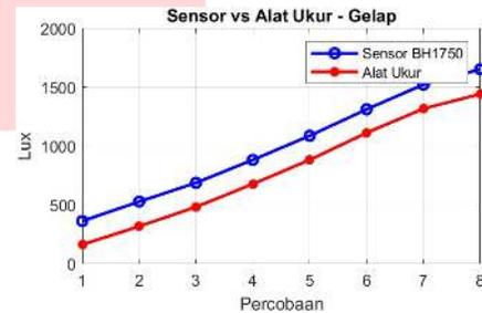
Figure 12 Grafik Sensor Vs Alat Ukur Kondisi Gelap
