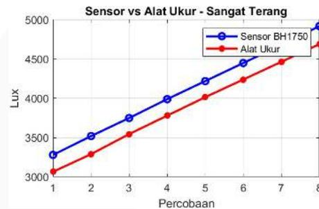
Figure 9 Grafik Sensor Vs Alat Ukur Kondisi Sangat Terang
