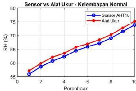
Figure 7 Grafik Sensor Vs Alat Ukur Kelembapan Normal
