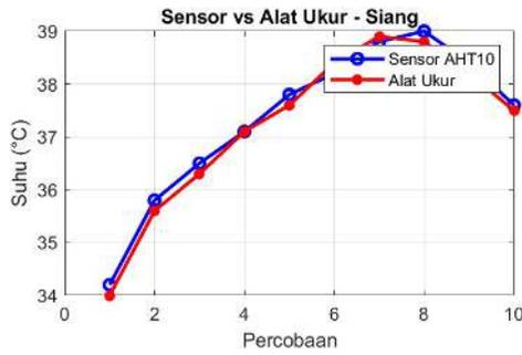
Figure 4 Grafik Sensor Vs Alat Ukur Siang
