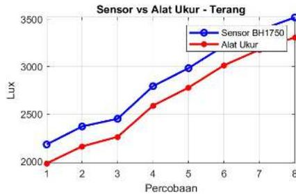
Figure 10 Grafik Sensor Vs Alat Ukur Kondisi Terang
