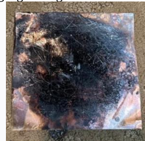
Gambar 4. 4 Efek Korosif NaOH
